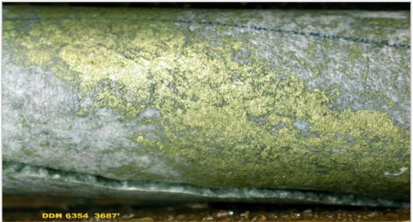
Figure 7-8: Drill Core Photograph Showing Chalcopyrite Mineralization
